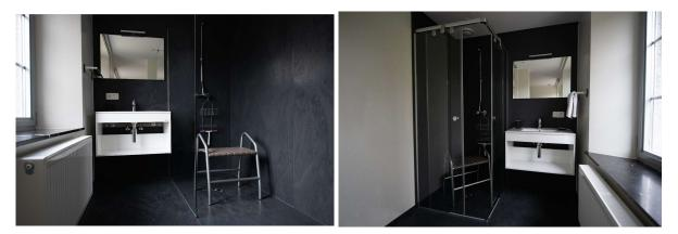
Despite the wooden floor, the flush-to-floor showers in the Sourmont Abbey could be implemented with wedi elements. The built-in shower element and the walls were then covered with the carbon black design surfaces of the wedi Top Line.
