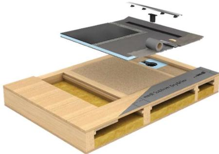
The drainage sits between beams in the installation void with the shower element placed precisely on top.
